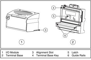
Figure 1. Installing the FP-PWM-520
